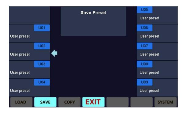
B. Click on the encoder button corresponding to any preset, and the preset name window and the entry keyboard will pop up. Rotate INPUT encoder to modify name, and click on OK to save them. The storage time is related to storage parameter value. The more parameters are saved, the longer the storage time is. Parameters are saved only after corresponding preset name is modified.
