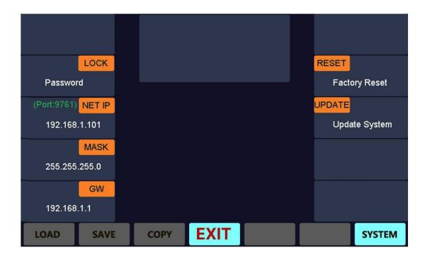
5. Click on the encoder button corresponding to Update System to enter the USB flash disk upgrade interface. All updatable data packets in the USB flash disk are automatically searched and displayed on the operation interface. Rotate the encoder to select the bin file of the data package to be upgraded and click on OK to start upgrading.
