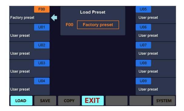
B. Click on corresponding encoder button to select a preset. Click on OK and the equipment will display the progress bar. The message bar will display a new preset name after call.
